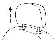
2. Simultaneously press and hold both the adjust/release button and the unlock/remove button, then pull up on the head restraint.
